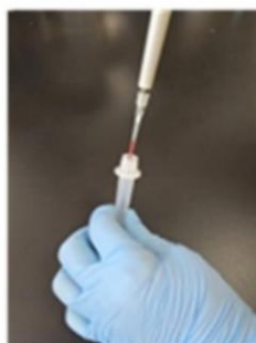
① Mixing chelex-100 solution with sample
