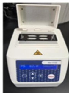
⑤ LAMP reaction at 62°C, 30min
